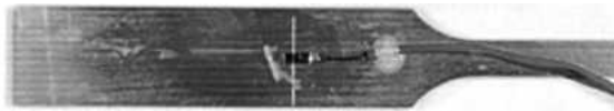
Fig. 2 Tensile specimen with an adhesive bonded strain gauge at the region with no waist. This enables the strain gauge to be used as load signal.
